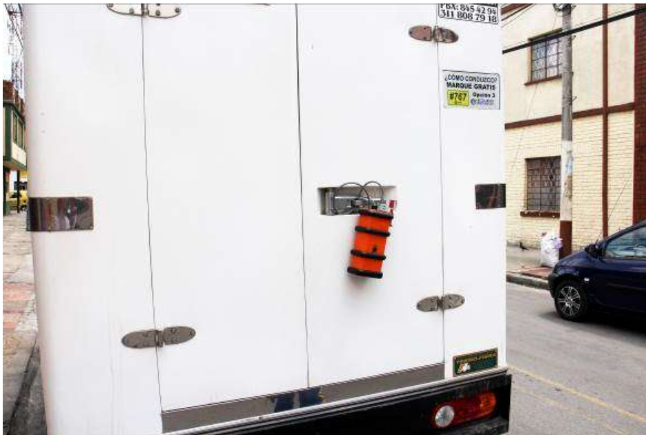
Figure 12: Hanging the Seal from the Truck Door Handle
