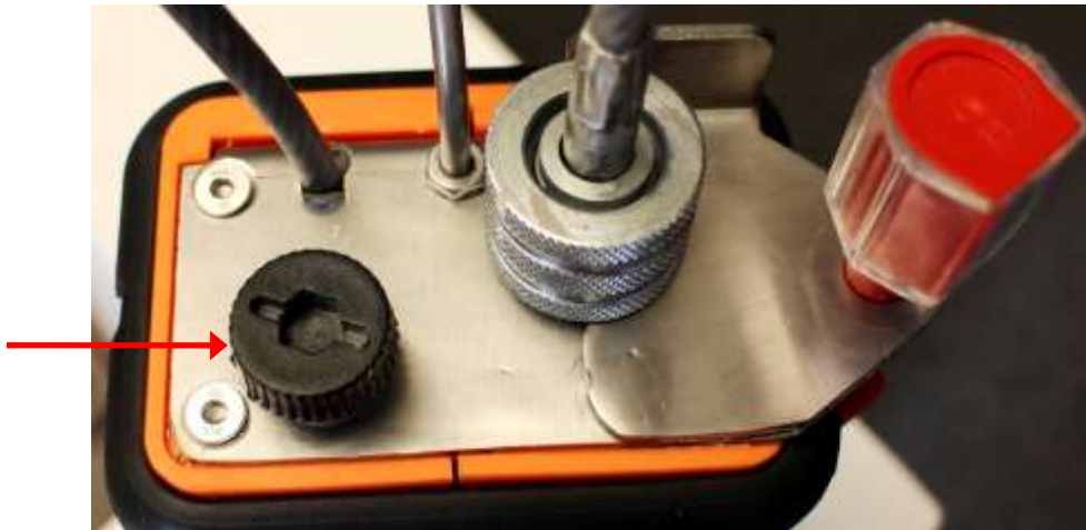
Figure 13: Charging the CelloTrack Battery
