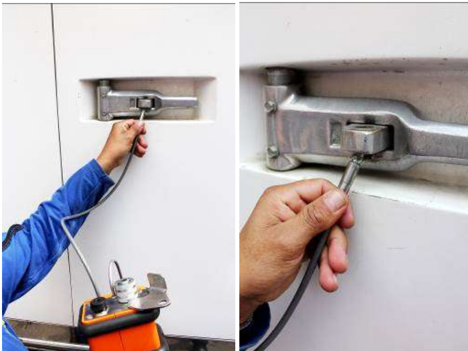
Figure 9: Passing the Wire Rope through the Truck Handle Bar
