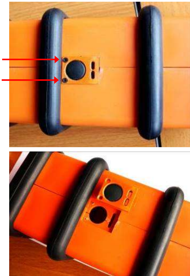
Figure 3: Removing the Operating Button and LED Window
