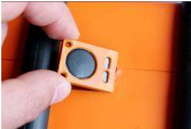
Figure 7: Install the Operating Button and LED Window
