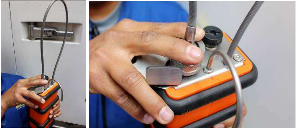
Figure 8: Detaching the Wire Rope
